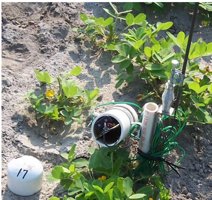
Figure 4. To overcome the range issue, the original mote antennas were enclosed in an 8 foot, 0.25 inch diameter hollow, flexible, fiberglass rod. The rods were mounted to a PVC pipe used as a supporting stake with a spring used for conventional CB antennas. The pipe also supported the PVC enclosure housing the node circuitry including the Mica2 motes.
