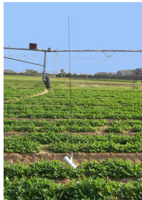
Figure 4. To overcome the range issue, the original mote antennas were enclosed in an 8 foot, 0.25 inch diameter hollow, flexible, fiberglass rod. The rods were mounted to a PVC pipe used as a supporting stake with a spring used for conventional CB antennas. The pipe also supported the PVC enclosure housing the node circuitry including the Mica2 motes.
