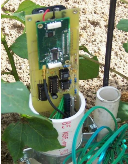
Figure 3. A sensor node's circuit board pulled part-way out of its PVC enclosure. The green circuit board is the mote. The node circuitry is powered by two alkaline AA batteries mounted to the back side of the sensor acquisition board.
