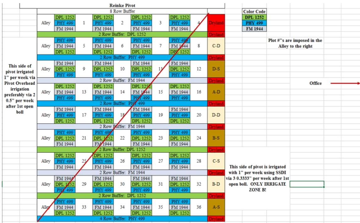
Figure 1. Randomized strips in the split field for the overhead and SDI irrigation treatments.
